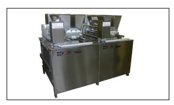
Modern two-component forming - extrusion ma hine with roller-gear system of deposition, for professional formation of zephyr, soft cookies, aerated fruit candy, aerated quark cheese and other confectionery & dairy masses of average viscosity.
